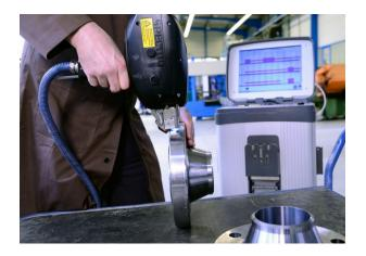
Spectral analysis is pivotal in determining the chemical composition of <u>metallic materials</u>, enabling precise identification and verification. At Applus+ Laboratories, we specialise in comprehensive spectral analysis services that ensure the traceability and integrity of your materials. By preventing material mix-ups, we help you avoid significant damage, especially in sensitive and security-relevant areas.
