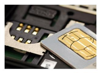
Secure Elements (SE) are a chip-based solution for mobile payment that enables secure storage of payment transactions and other sensitive credentials. Secure Elements in any of their form factors USIM cards (UICC), Embedded SE (eSE), SD cards or add-ons are one of the most secure and reliable solutions for NFC payments market.
