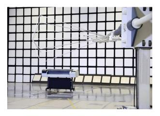
In order to allow the coexistence of different electrical and electronic products within the same environment their electromagnetic compatibility must be ensured, avoiding any interference between the different equipment that may lead to malfunctions. Electromagnetic compatibility validation is a mandatory requirement for electrical and electronic product comercialitzation in international markets.
