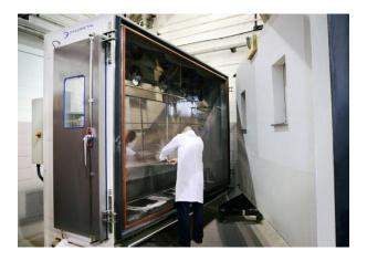
Manufacturers of construction products should ensure that the materials used are functionally operational throughout the building's lifetime. Before launching a new product in the market, they should evaluate how it will behave when faced with cycles that accelerate the operating conditions to which it will be subjected.
